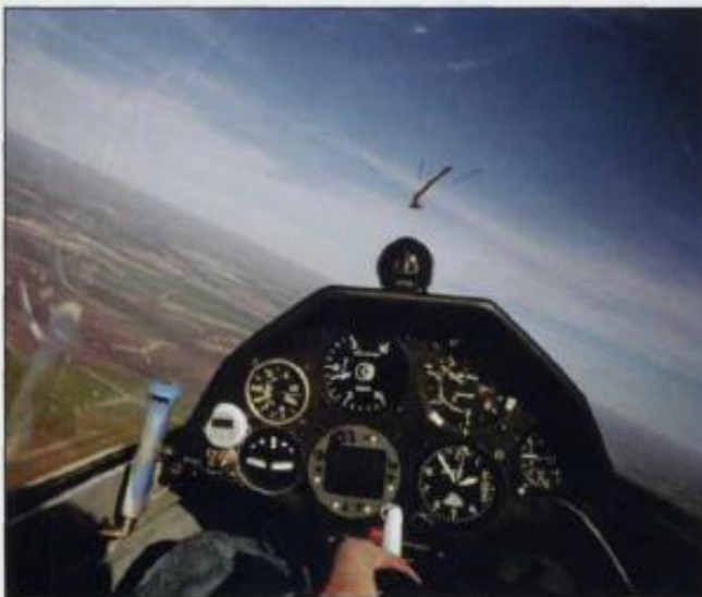
Author's Ventus A cockpit view during a properly coordinated left turn at 43 kts, with yaw string at about 10 degrees on the high side during this relatively gentle turn.
