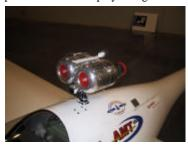
sailplane with a pair of jet engines for thrust. As I can attest, it wasn't so "silent" anymore.
