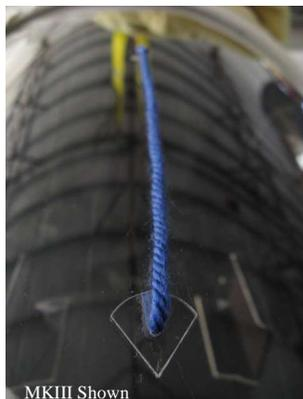
The Bumper MKIV high tech Yaw String features a wool or acrylic string in multiple colors mounted to a clear and aerodynamic pad. Because the mounting pad is totally transparent, you might be surprised how irritating the standard "piece of gap tape" method really is. One less thing to block your field of vision.
