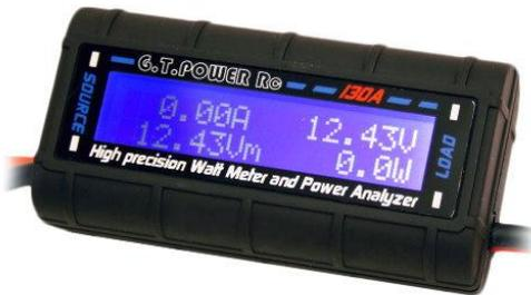
This inexpensive (about \$30) and small (85x42x25 mm and 82g) device displays both real time voltage (to 60Vdc), current (to 130A) and wattage – plus measurements over time of amps, volts and watts (see details below). Cool!
